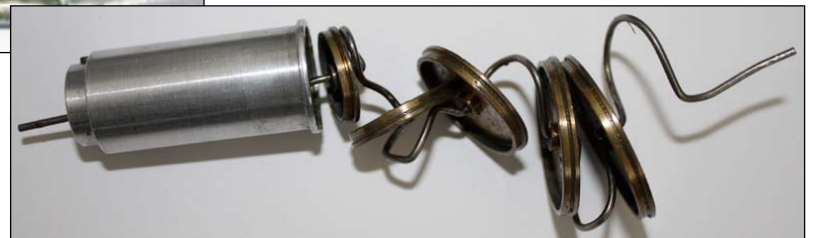
Bent drilling needle in telescope guidance of an IML-RESI M300
