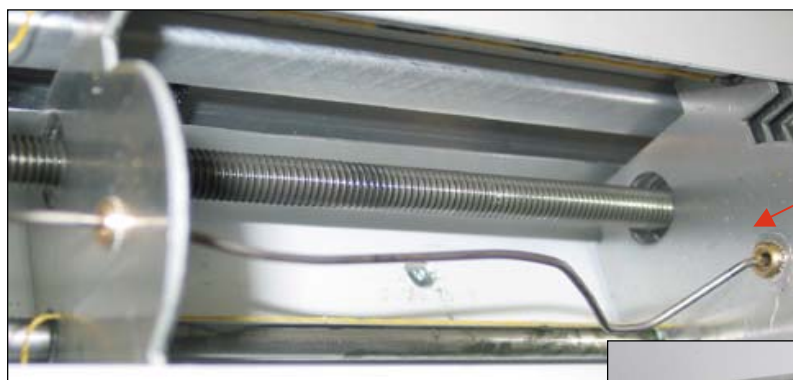
Bent drilling needle in telescope guidance of an IML-RESI M300
